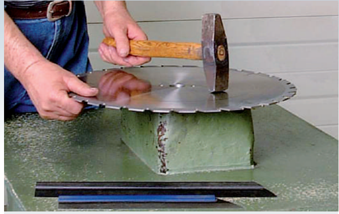
Feinrichten · High-precision straightening of the blades
