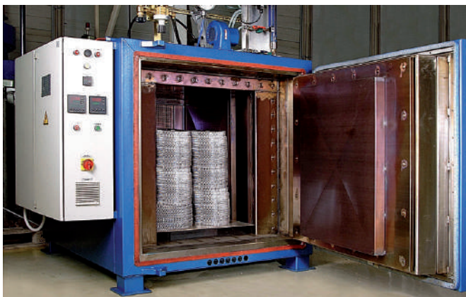
Anlassofen · Tempering furnace
