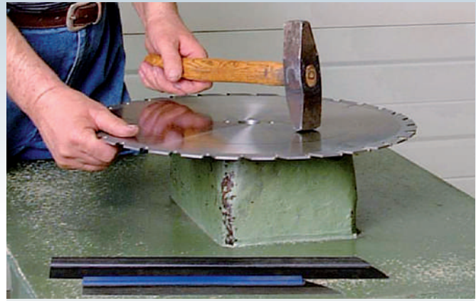
Feinrichten · High-precision straightening of the blades
