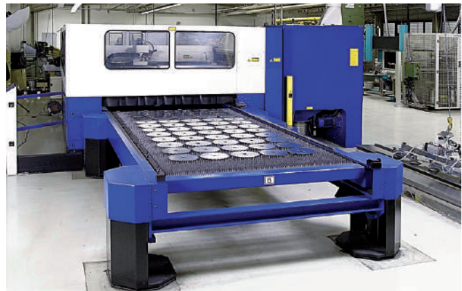
Feinrichten · High-precision straightening of the blades
